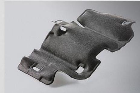
Highly efficient combustion engines require state-of-the-art heat insulation. Due to its superior thermomechanical stability, Acrodur is the perfect enabler for turning natural fibers into encapsulation parts. An additional benefit is the acoustic noise reduction. Acrodur can also be applied in other exterior parts, such as underbody shields.
