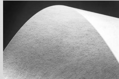
Glass fiber nonwovens are used as support layers for vinyl and carpet flooring tiles or for bituminous roofings. Further applications include robust wall coverings and facing layers for mineral wool mats, construction boards or fiber-reinforced plastic parts.
