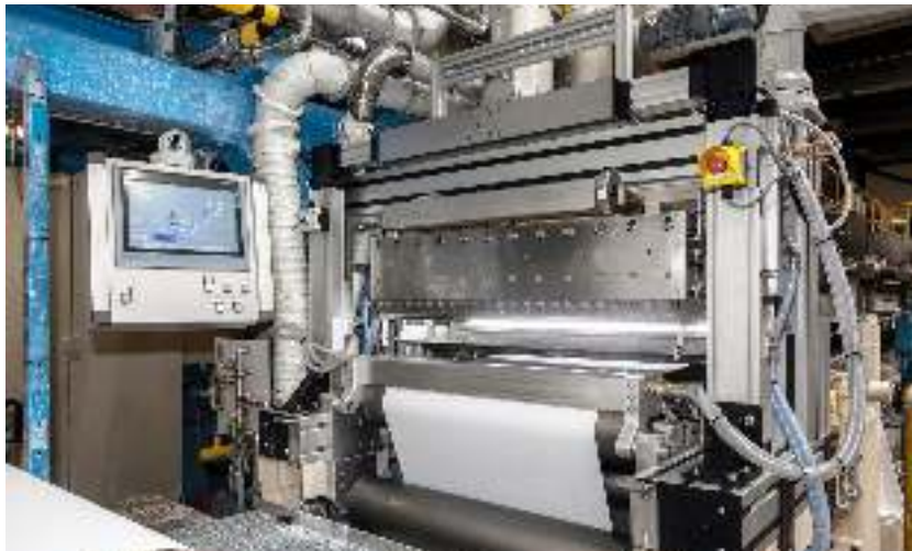
BASF has added a curtain coater to its pilot coating facility
